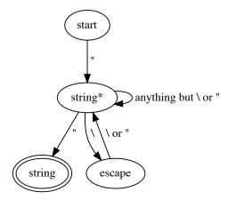
Figure 1: A finite-state machine for lexing a Scheme string.
